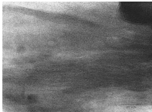
Figure 13 High-resolution TEM image of a C-15A/PP nanocomposite.
