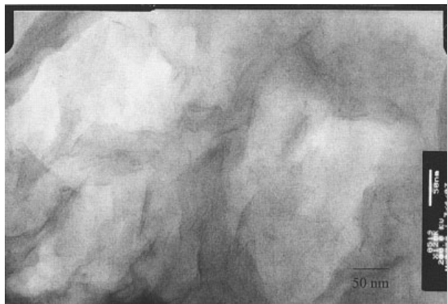
Figure 11 High-resolution TEM image of a C-15A/PP nanocomposite.
